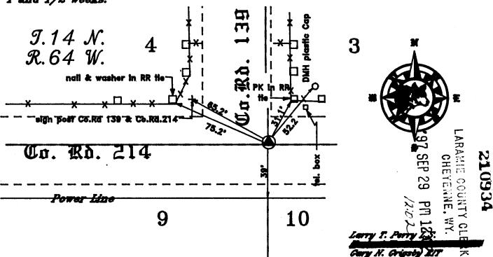
Note: Rebar with Aluminum Cap set 40.00' North for W.C.
